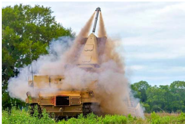
An Assault Breacher Vehicle (ABV) launches an inert Mine Clearing Line Charge during obstacle reduction training.
